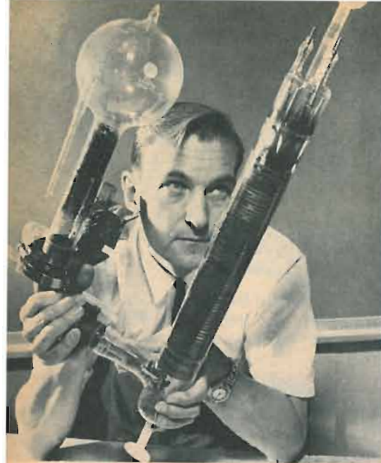
RCA sun bottle: First gas lasers to produce intense rays of ultraviolet light continuously up to 1000 hours, to be used to solve mysteries of life.
