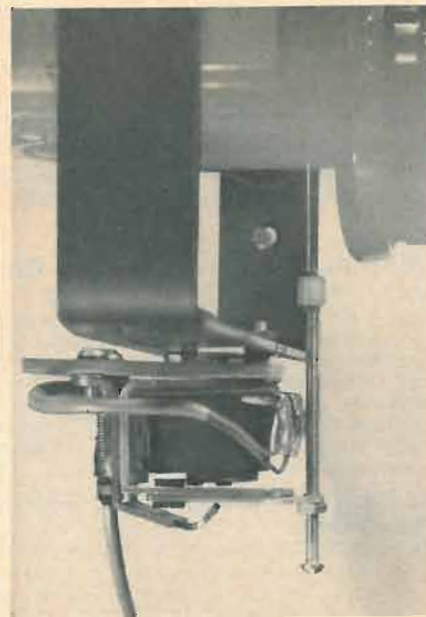
Fig. 8—Relay and extension arm mounted ready to trigger a spring-drive camera.
