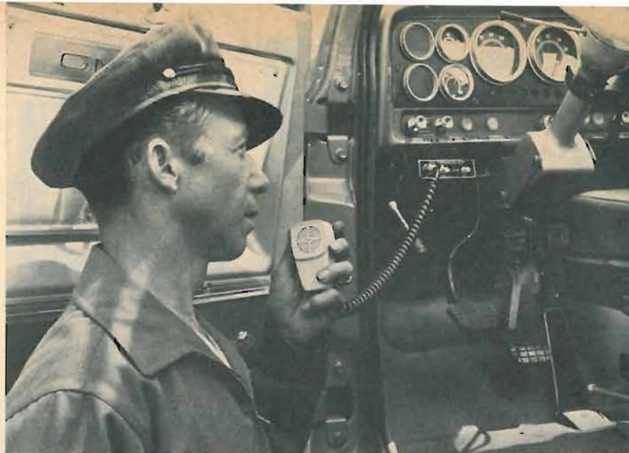
CB hits the road: Truck users will soon be able to buy GMC trucks equipped with factory-installed CB transceivers and antennas. Units are smaller than a cigar box. Communications gear will be supplied by Lafayette Radio Electronics Corp., to GMC Truck & Coach Division.
